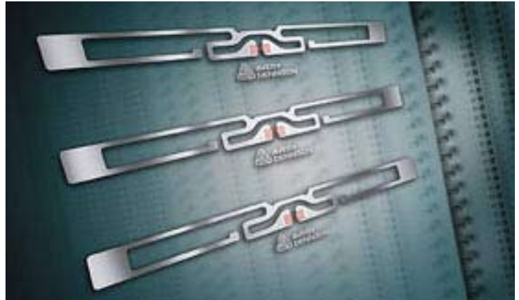
EPC-compliant RFID tag inlays, designed for high performance and high-volume labeling, are converted into labels and are enclosed with Alliance's small order.
