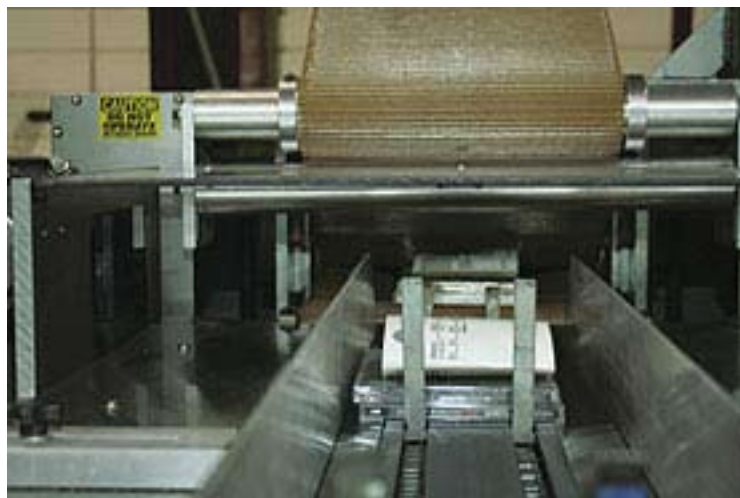
Stacked products comprising a small order, complete with return-policy and RFID-enabled labels, convey into one of two cohesive package-forming machines at Alliance Entertainment.
