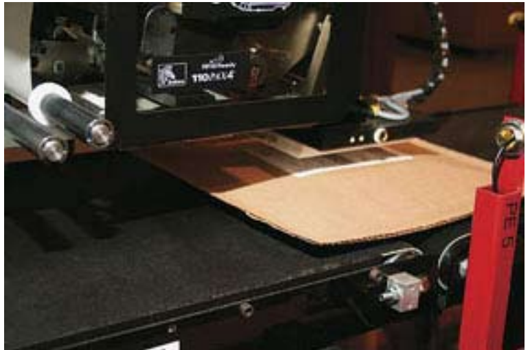
A printer/applicator affixes a bar-coded shipping label to the outside of a package. The label data corresponds to data encoded on the inner RFID label.
